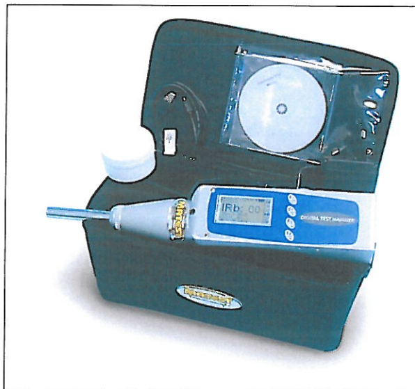
Sclerometrul Digital MATEST C386N
